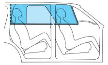
**WARNING:** If the Safety Canopy<sup>®</sup> System has deployed, the Safety Canopy<sup>®</sup> will not function again unless replaced. The Safety Canopy<sup>®</sup> System (including the A, B, C, and D pillar trim and headliner) must be inspected and serviced by an authorized dealer. If the Safety Canopy<sup>®</sup> is not replaced, it will not function again, which will increase the risk of injury in a future collision.
